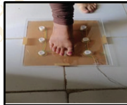
Fig 14(c): Stress applied on piezoelectric devices
